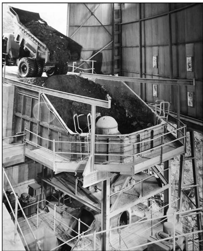
Figure 11. The primary crusher at Bardon Hill Quarry, date unknown. (Photo: Aggregate Industries Archive)
